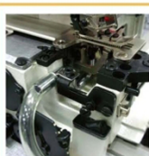
Lint removal pipe
